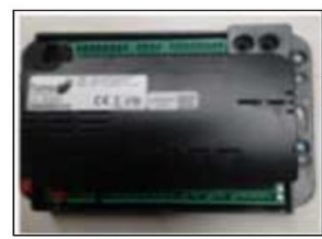
Model: Fumis Alpha 85-230-80x Type: Palazzetti 002820700 Input: 230 V, 50/60 Hz, 3 A max
